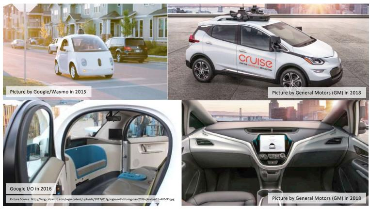
Highest level of autonomous driving (Level 5 of 5), where a car can drive from A to B without human supervision.
