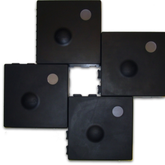
Figure 2: Four tangible tiles assembled into a playground. The light output is placed in the upper right corner of the tile while the “bump” indicates the position of the force sensor.
